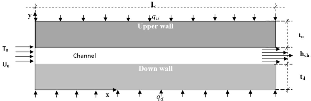
Fig1. Geometric configuration of microchannel heat sink.
