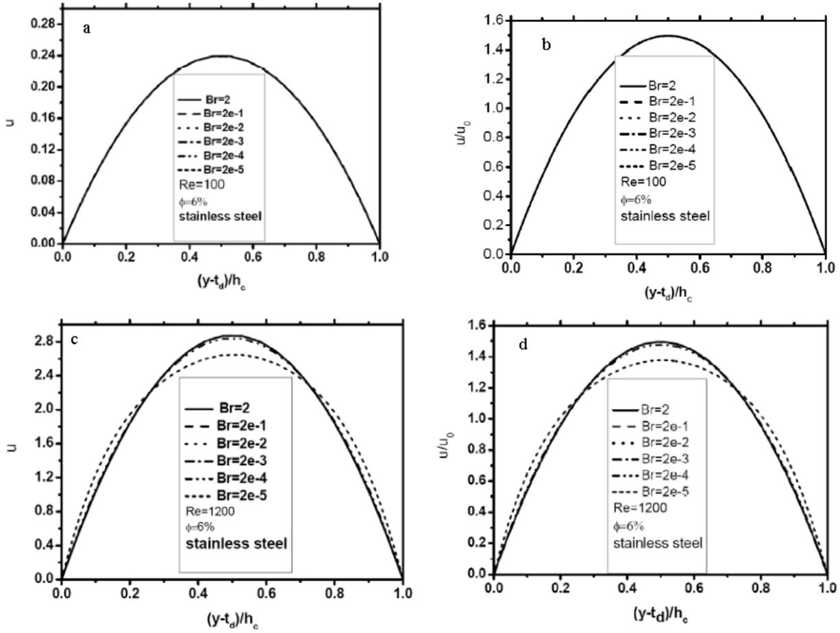
Fig. 4 Dimensional and dimensionless fully developed velocity profile.
