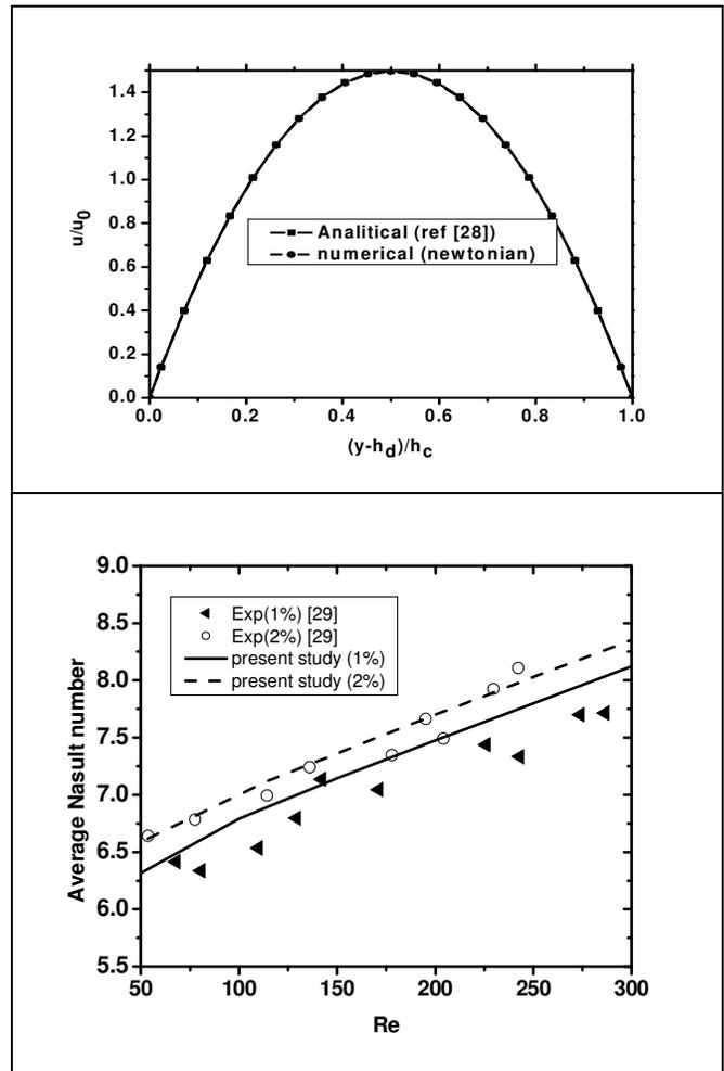
Fig. 3 comparison with the experimental results (a) analytical solution [28].(b) experimental data [29].
