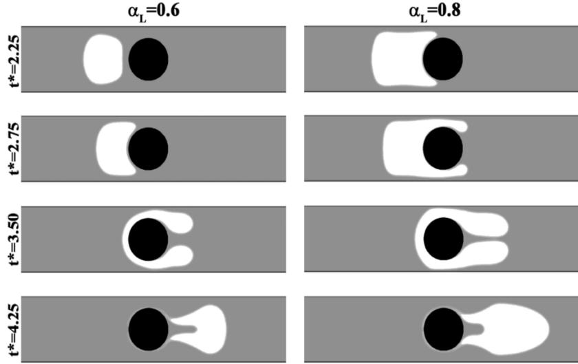
Fig. 8. Effect of the ratio of the droplet size to channel width,  $Ca=0.00085$ ,  $\alpha_D=0.6$
