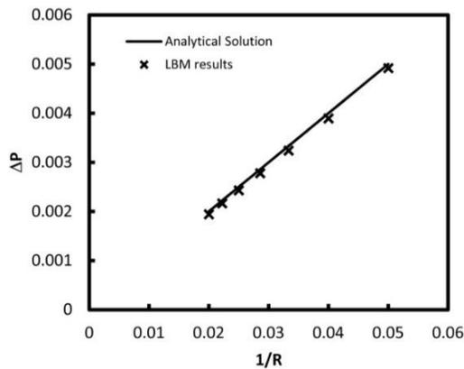
Fig. 1. Pressure difference between inside and outside of a droplet versus curvature
