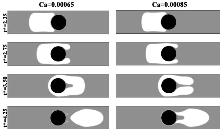
Fig. 5. Effect of Capillary number,  $\alpha_D=0.6$ ,  $\alpha_L=0.8$
