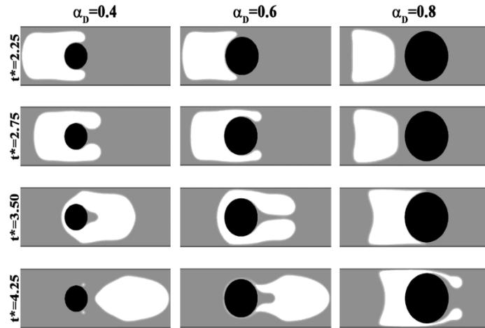
Fig. 7. Effect of the ratio of the particle size to channel width,  $Ca=0.00085$ ,  $\alpha_L=0.8$
