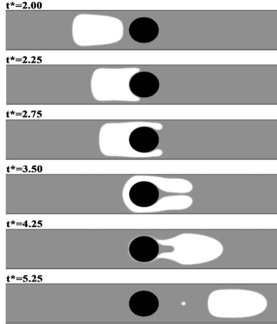
Fig. 3. Transient interaction,  $Ca=0.00045$ ,  $\alpha_D=0.6$ ,  $\alpha_L=0.8$
