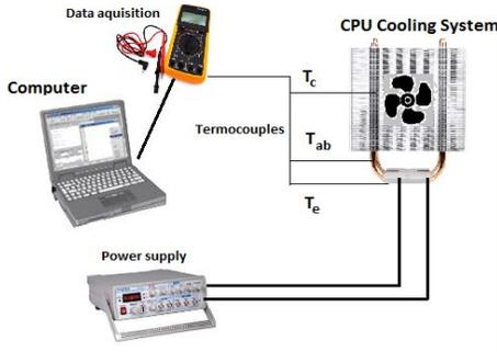
Fig. 4. Schematic of the setup
