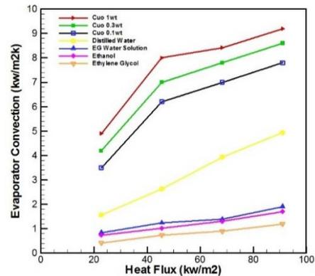
Fig. 11. Convection coefficient in evaporator
