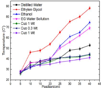
Fig. 7. Distribution of temperature along the heat pipe for 25 Watts
