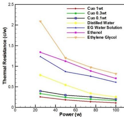
Fig. 13. Thermal resistance diagram of the whole heat pipe
