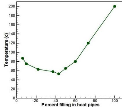
**Fig. 6.** Temperature Vs fluid filling percentage in heat pipe for 25 watts
