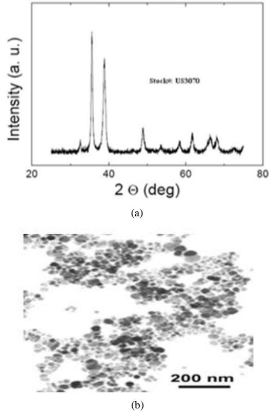
**Fig. 1.** (a) X-ray diffraction spectroscopy copper oxide nanoparticles (b)Copper oxide nanoparticles by transmission electron microscopy
