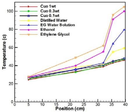
Fig. 8. Distribution of temperature along the heat pipe for 50 Watts
