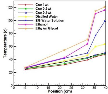
Fig. 9. Distribution of temperature along the heat pipe for 75 Watts
