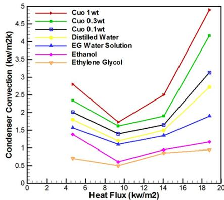
Fig. 12. Convection coefficient in condenser
