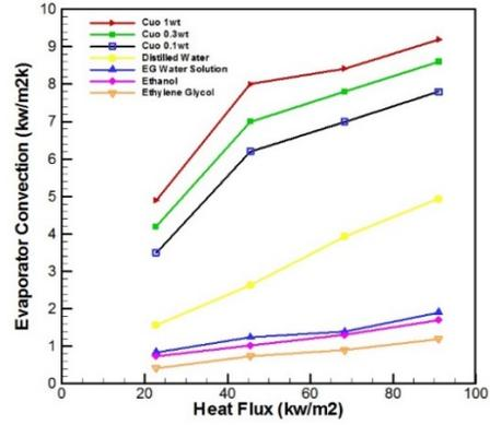
Fig. 5. Convection coefficient in evaporator
