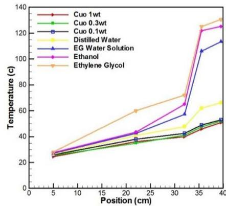
Fig. 10. Distribution of temperature along the heat pipe for 100 watts
