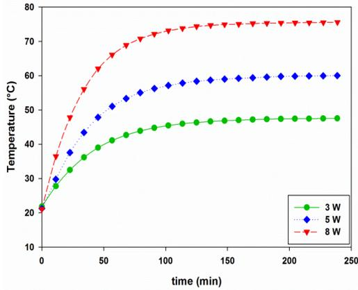
Fig. 2. Temperature-time profile of unfilled heat sink
