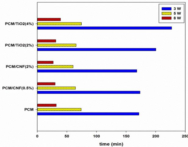
Fig. 6. Melting completion time for PCM, PCM/CNF and PCM/TiO<sub>2</sub>
