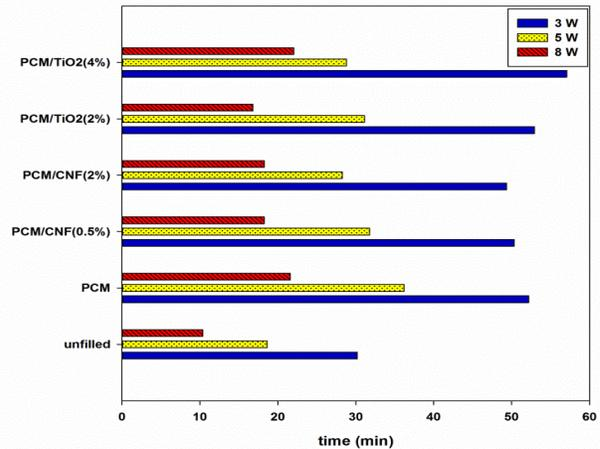
Fig. 5. Comparison of operating times to reach 35°C for various particle loadings and power level
