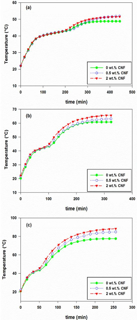
Fig. 3. Temperature-time profile of the PCM/CNF heat sink for power level of (a) 3W (b) 5W (c) 8W
