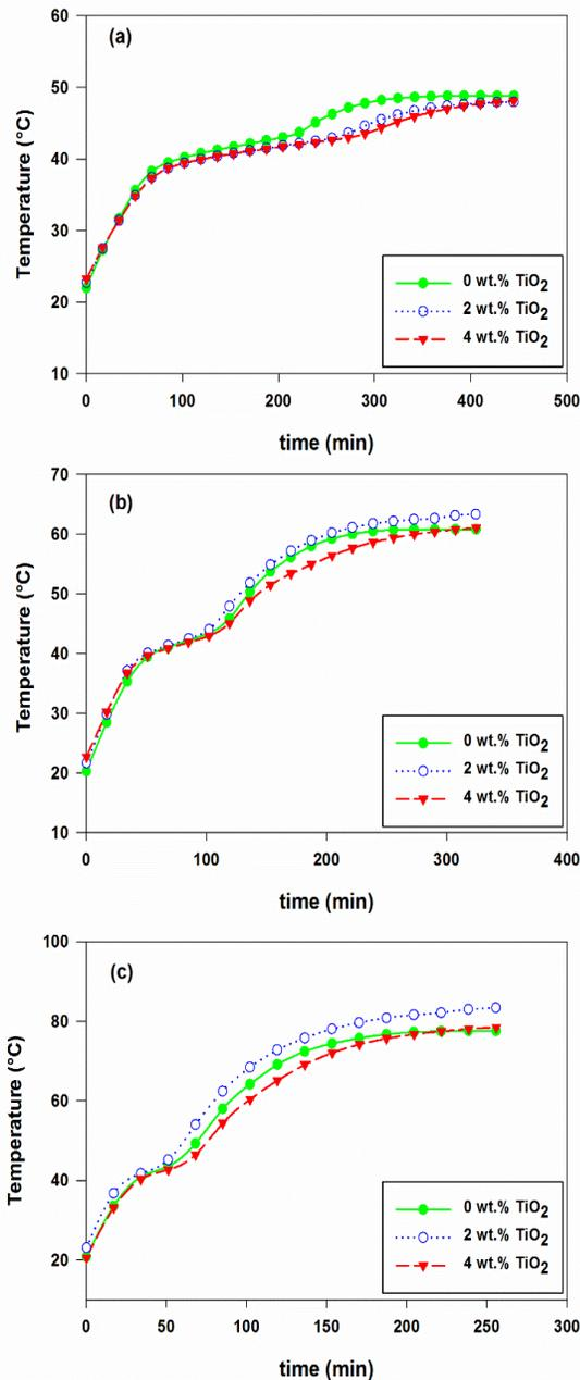
Fig. 4. Temperature-time profile of the PCM/TiO<sub>2</sub> heat sink for power level of (a) 3W (b) 5W (c) 8W
