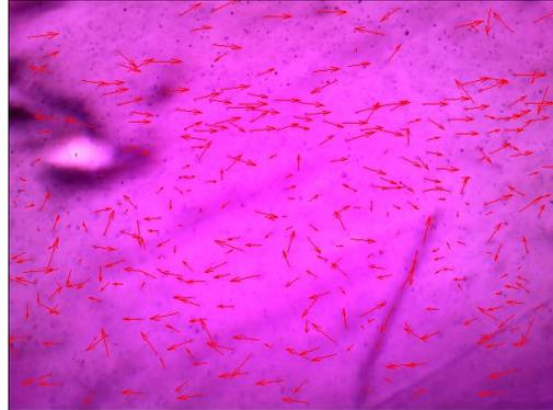
Fig. 6. Particle motion vectors, in laser-on mode at the beginning of the channel
