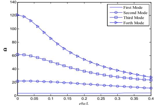
**Fig. 3.** First frequency of C-F nano-column with various nonlocal elasticity ( $\eta=1$ )
