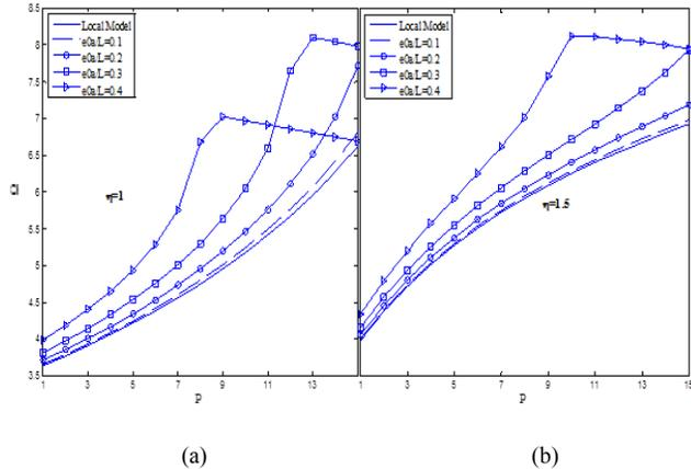
**Fig. 2.** Non-dimensional frequency parameter of C-F nano-column with various P (a:  $\eta=1$ , b:  $\eta=1.5$ )
