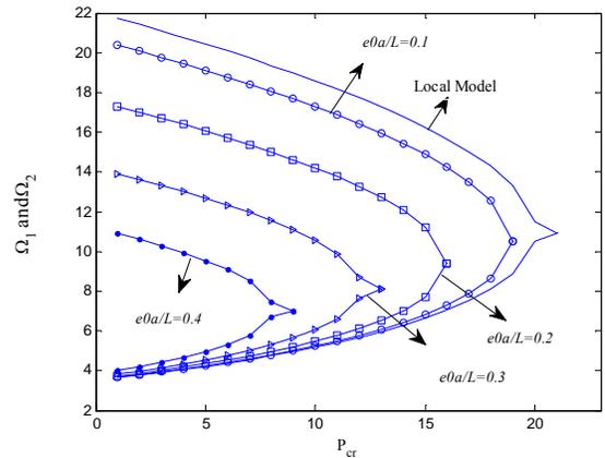
**Fig. 4.** First and second frequency of C-F nano-column with various P ( $\eta=1$ )
