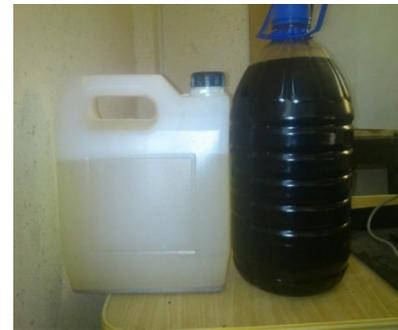
Fig. 4. Pure oil and Ag-oil nanofluid at 0.12% wt. prepared by E.E.W technique
