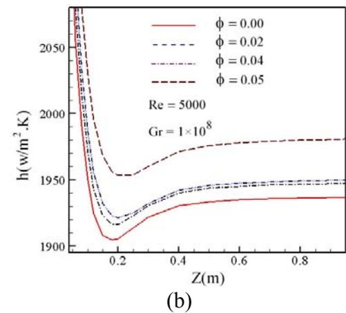
**Fig.9.** Variation of the convective heat transfer coefficient along the tube length with different Grashof number for  $\text{Al}_2\text{O}_3$ -water nanofluid, nanoparticle volume concentration of 0, 0.02, 0.04 and 0.05 and Reynolds number of 5000.
