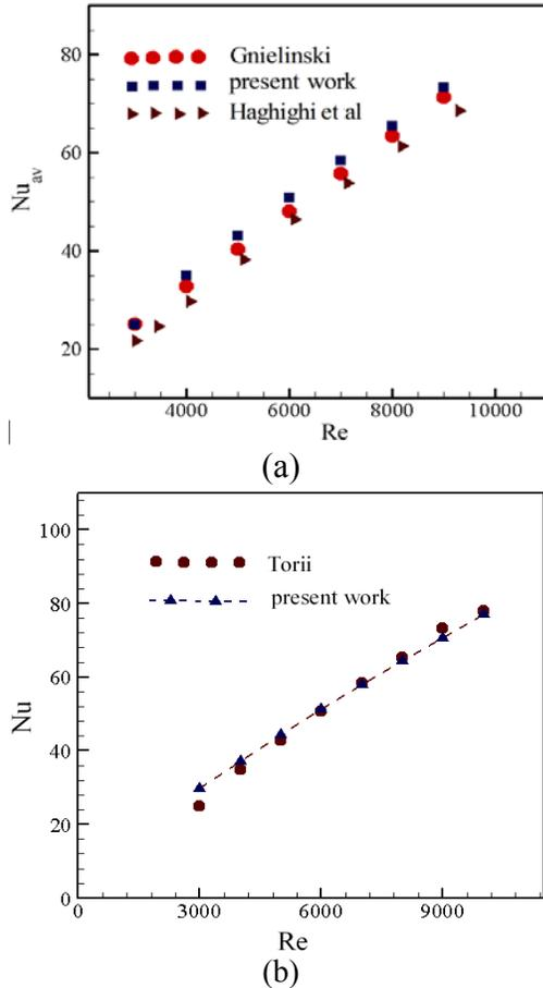
**Fig. 3.** a) Comparison of the axial evolution of Nu in a horizontal tube with the results obtained by Gnielinski [48] and Haghghi et al [49], b) Comparison of the axial evolution of Nu in a horizontal tube with the experimental results obtained by S. Torii [50].
