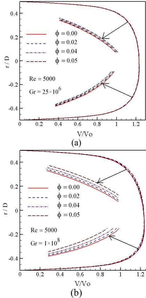
**Fig. 4.** Variation of the dimensionless fully developed axial velocity profiles with different Grashof number for  $Al_2O_3$ -water nanofluid, nanoparticle volume concentration of 0, 0.02, 0.04 and 0.05 and Reynolds number of 5000.
