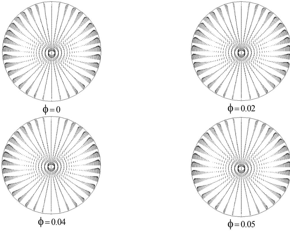
**Fig.6a.** Effect of nanoparticles concentration on the Vectors of secondary flow for different volume fraction at  $Gr = 25 \times 10^6$
