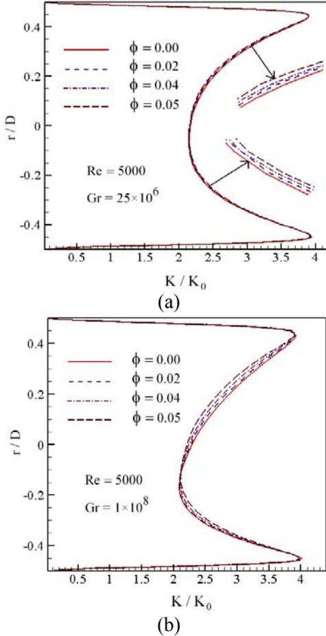
**Fig. 5.** Variation of the dimensionless fully developed turbulent kinetic energy profiles with different Grashof number for  $Al_2O_3$ -water nanofluid, nanoparticle volume concentration of 0, 0.02, 0.04 and 0.05 and Reynolds number of 5000.
