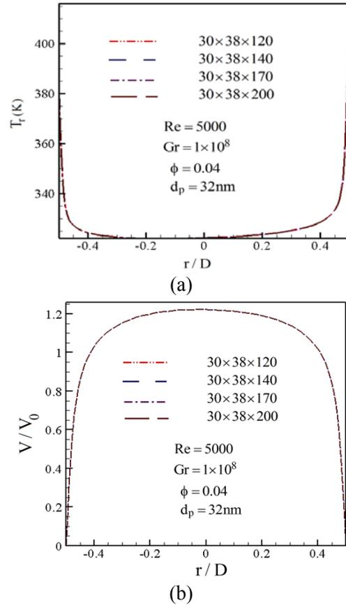
**Fig. 2.** Grid independence test: (a) fully developed temperature (b) centerline axial velocity
