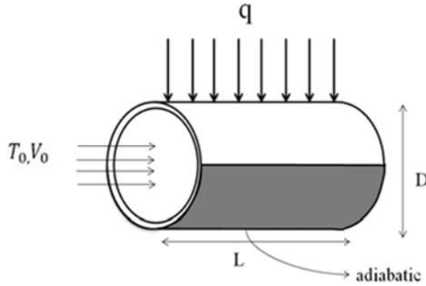
**Fig. 1.** Schematic of the considered horizontal tube
