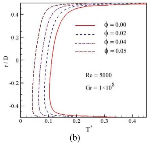
**Fig. 7.** Variation of the dimensionless fully developed temperature profiles with different Grashof number for  $\text{Al}_2\text{O}_3$ -water nanofluid, nanoparticle volume concentration of 0, 0.02, 0.04 and 0.05 and Reynolds number of 5000.
