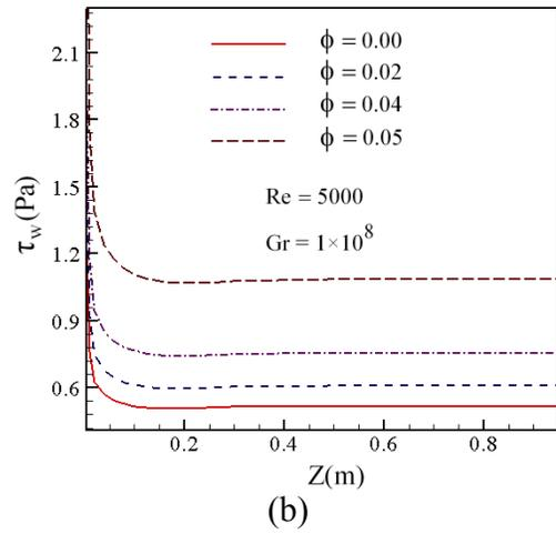
**Fig. 8.** Variation of the shear stress along the tube length with different Grashof number for  $\text{Al}_2\text{O}_3$ -water nanofluid, nanoparticle volume concentration of 0, 0.02, 0.04 and 0.05 and Reynolds number of 5000.
