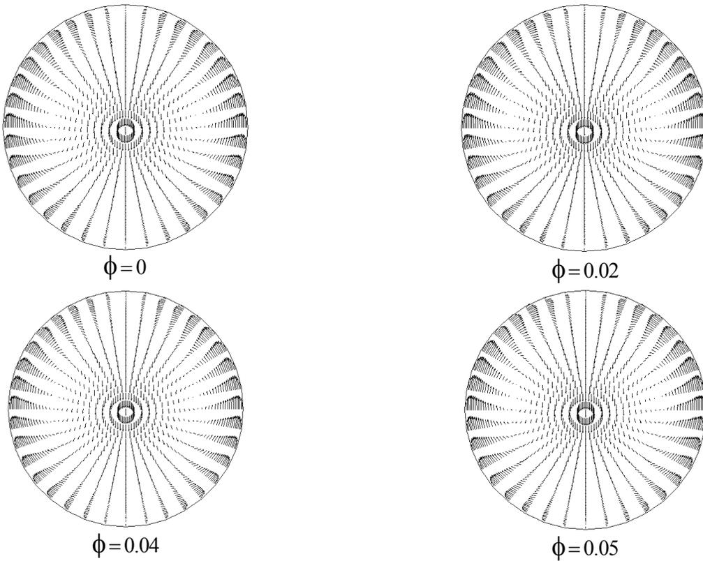
**Fig.6b.** Effect of nanoparticles concentration on the Vectors of secondary flow for different volume fraction at  $Gr = 1 \times 10^8$
